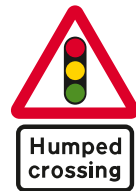
Signal-controlled pedestrian crossing on a road hump
